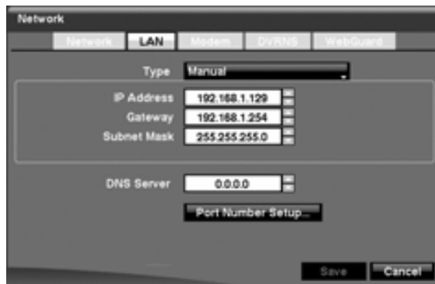
Figure 3-25 LAN (Manual) Setup Screen
